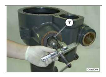
Take the bevel pinion out of its housing, by beating with hammer made of soft material on the splined end.
