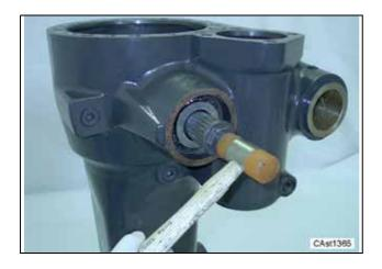
10. Once the bevel pinion (2) has been removed, collect shims (9) and spacer (8).
