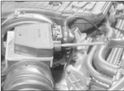
11.16 Adjusting the mixture (CO) setting - 2.0 litre 16-valve models
