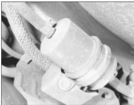
25.3 Fuel filter showing mounting and hose connections
