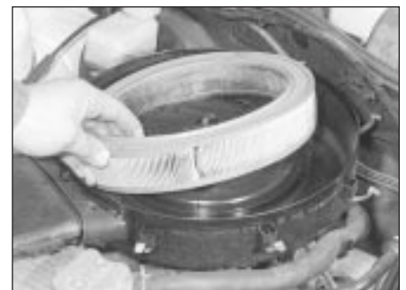
24.2b . . . and withdraw the filter element
