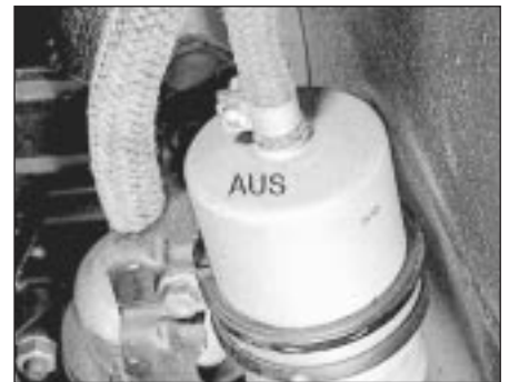
25.4 Fuel filter directional marking
