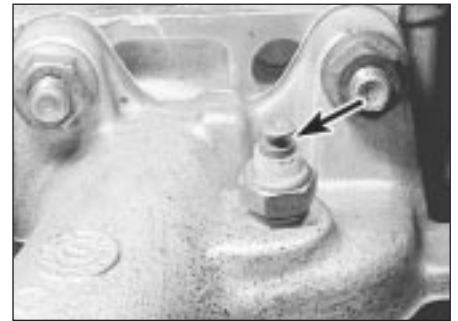
32.19b On 1.3 litre models, unscrew temperature gauge sender unit from the manifold to bleed the cooling system
