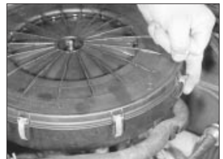
24.1b . . . and release the retaining clips . . .
