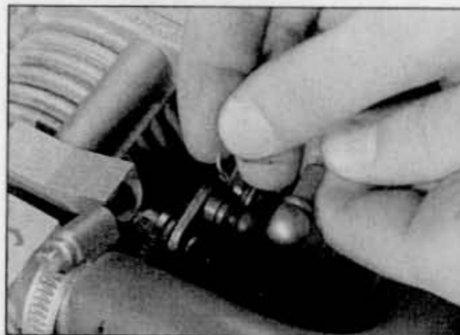
19.2 Disconnecting the throttle cable end from the throttle valve lever - SOHC model
