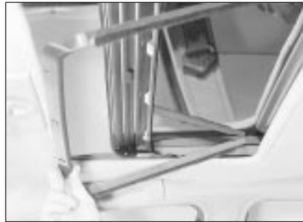
34.2B . . . and withdraw the guide rail plastic surround
