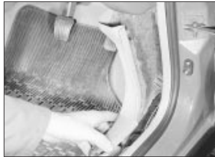
36.5 Removing the driver's footwell side trim panel
