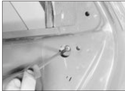
25.13A Remove the remaining securing screw . . .
