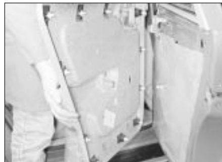
17.20 Removing a rear door inner trim panel
