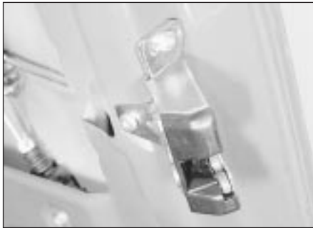
13.1 Tailgate lock (trim panel removed)
