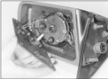
27.2 Removing the mirror glass - electric mirror (mirror removed)
