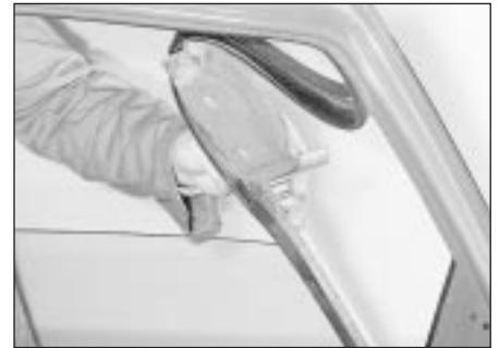
25.13B . . . then withdraw the guide rail from the door
