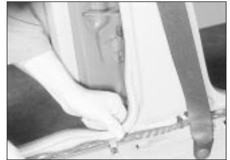
36.10 Pull the weatherstrip from the sides of the body pillar . . .
