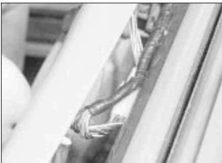
17.7 Mirror switch wiring connector in bracket at top of door
