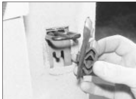
36.19A Removing the rubber stop from the seat catch
