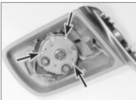
27.10 Mirror motor securing screws (arrowed)
