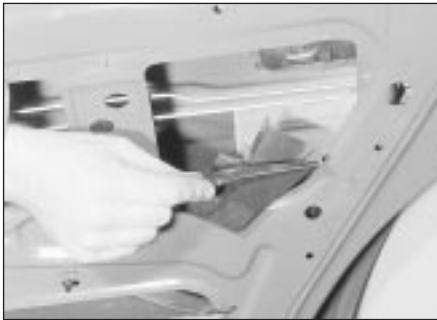
21.12 Unclip the plastic shield from the lock
