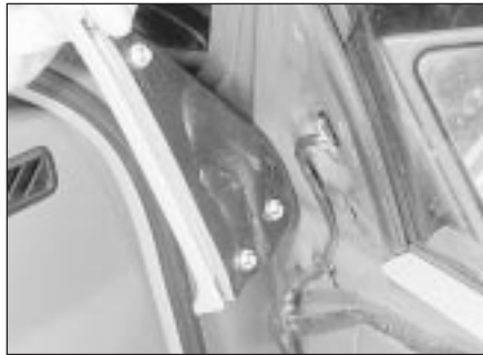
27.6 Removing the mirror trim panel . . .
