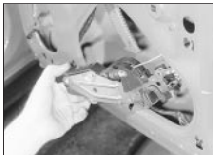
21.6 Removing the lock assembly - model with central locking
