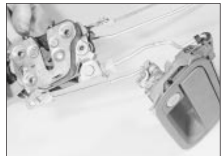
21.3 View of removed door lock and exterior handle assembly, showing operating rod attachments
