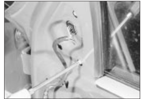
27.7A . . . for access to the mirror securing screws
