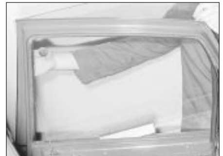
25.15 Withdrawing the window glass from the door
