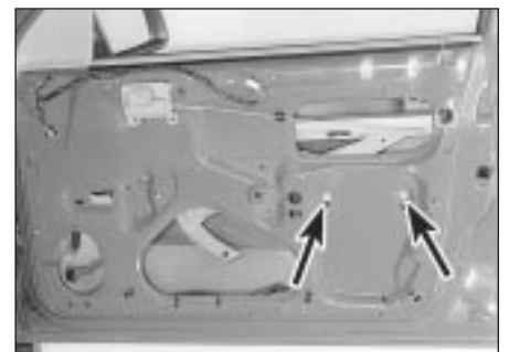
25.5 Window lower guide rail securing screws (arrowed)
