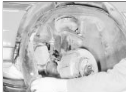
31.1 Removing a wheel arch liner
