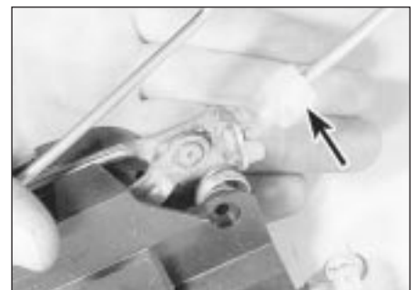
21.7 Exterior handle operating rod adjuster wheel (arrowed) at lock end of rod
