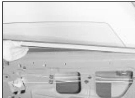
25.14 Pulling the inside weatherstrip from the window aperture
