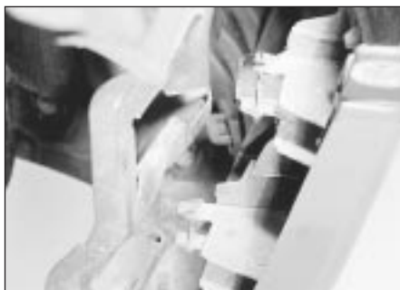
28.5 Front bumper retaining clips released from body
