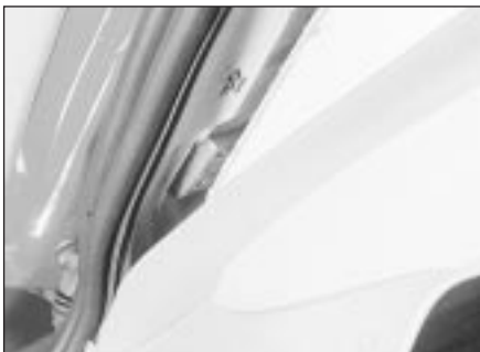
12.6A Prise off the rear roof trim panel . . .
