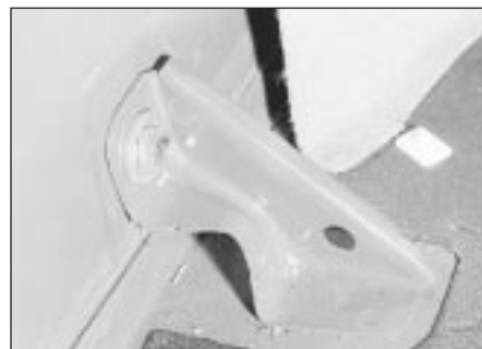
28.8B . . . to expose the bumper securing nuts
