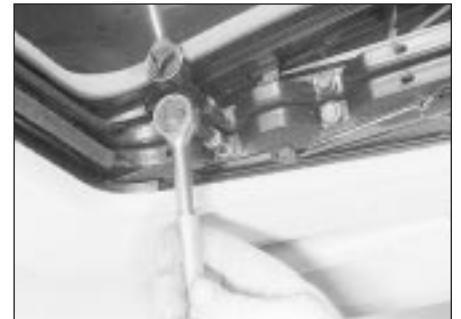
34.5 Loosening a glass panel securing screw
