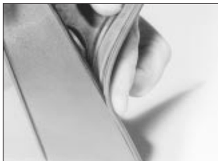
27.8 Locating the weather seal on the mirror housing
