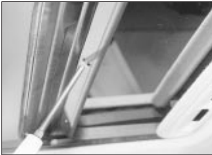
34.2A Extract the four securing screws . . .
