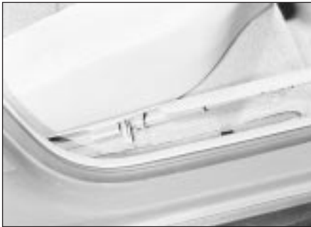
36.2 Sill trim panel removed to expose securing clips
