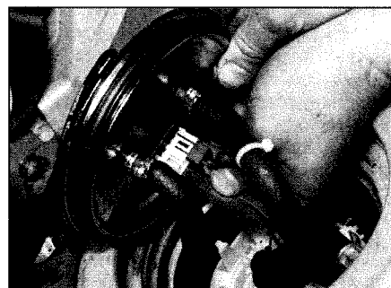
6.6 Disconnect the fuel gauge sender wiring plug
