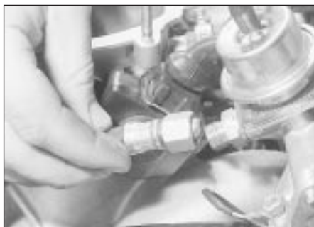
12.73 Disconnecting the fuel return line from the fuel pressure regulator
