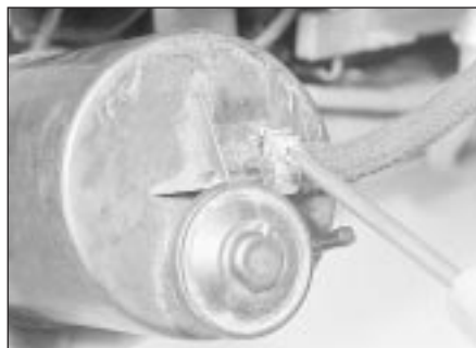
12.98b Disconnecting a hose from the canister
