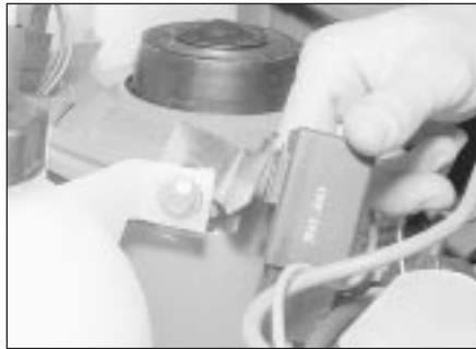
12.36a Removing the control relay and bracket
