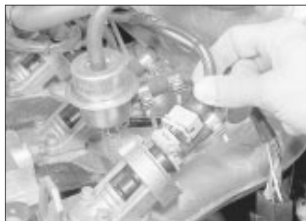
13.3b Disconnecting a fuel injector plug
