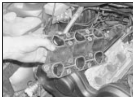
15.43 Removing the manifold flange
