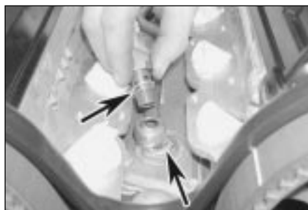
16.24b . . . then unscrew the union bolts and detach the pipes from the oil cooler (sealing washers arrowed)
