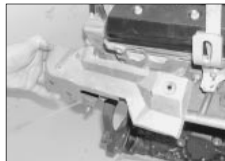
16.26b . . . and upper heatshields from the right-hand exhaust manifold
