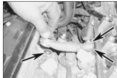
16.22 Unscrew the retaining bolts and remove the coolant outlet from the engine (sealing rings arrowed)
