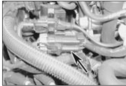
15.41 The injector wiring harness connector (arrowed) is clipped onto the engine rear lifting bracket (shown with engine removed)
