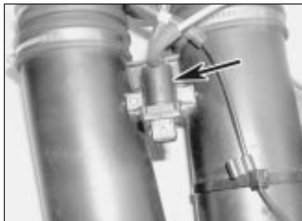
17.4 The intake duct switchover valve solenoid valve (arrowed) is mounted on the rear of the pre-volume chamber (shown with chamber removed)
