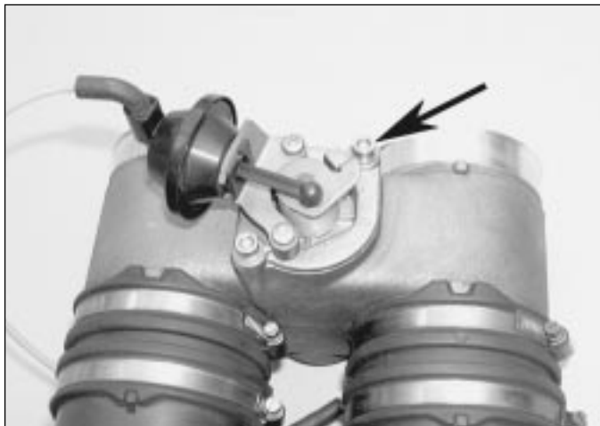
17.11 Undo the retaining screws (arrowed) and remove the switchover valve assembly from its housing
