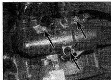
7.25a Thermostat housing retaining bolts - 2.2 litre petrol engine models
