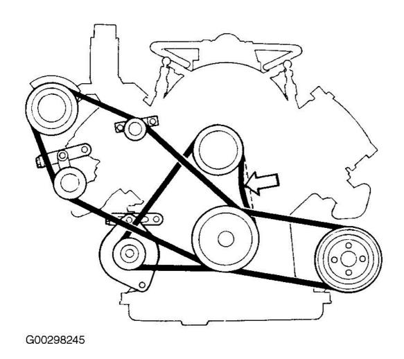
Fig. 2: Identifying Drive Belt Routing Courtesy of VOLVO CARS OF NORTH AMERICA.
