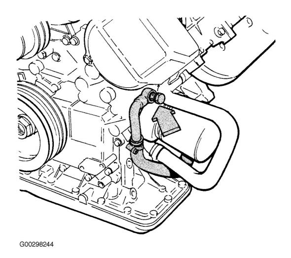
Fig. 1: Identifying Coolant Hose Banjo Bolt Courtesy of VOLVO CARS OF NORTH AMERICA.
