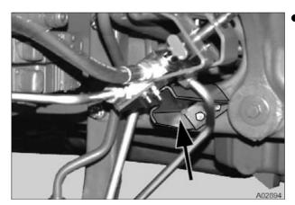
• Screw on bracket (arrowed) using M8x20 hexagon screws and spring washers.
