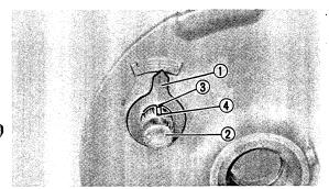
3. When installing the wear indicator plate ① to the camshaft ② align the projection ③ on the wear indicator plate with the slot ④ on the camshaft.
