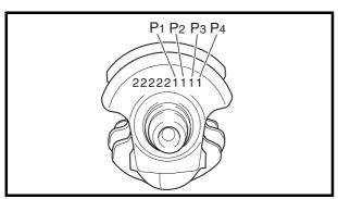
For example, if the connecting rod "P1" and the crankshaft web "P1" numbers are "5" and "1" respectively, then the bearing size for "P1" is:
