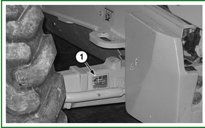
TX1107870A-UN: MFWD Front Axle Housing Serial Number Plate Location
