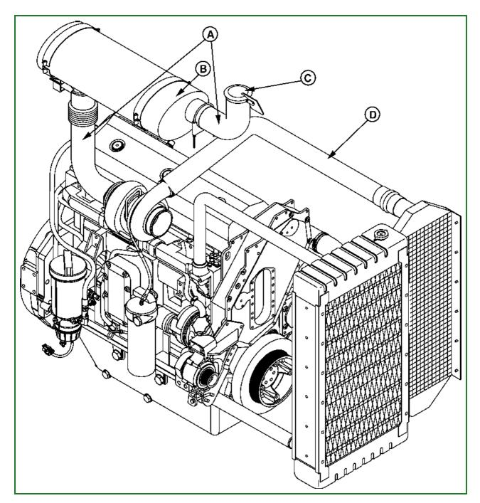
RG10660-UN: Check for Intake and Exhaust Restrictions
