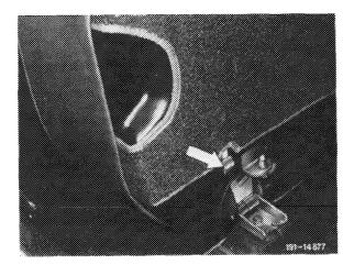
3 Push out cover at left and right adjacent to rear seat backrest by means of a plastic wedge.
