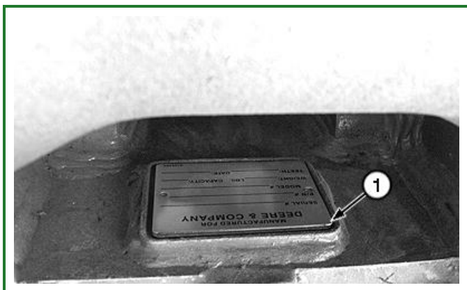
TX1017853A-UN: Hydraulic Coupler Serial Plate
