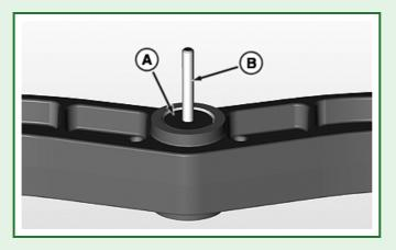
RXA0098301-UN: Removing Isolator and Pivot Bushing
