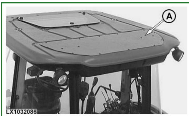
LX1032086-UN: Opening the Roof
